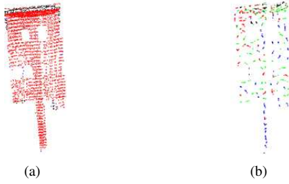
Fig. 6. Comparison of point classification result of a façade patch before and after smoothing. (a) shows the classification result without smoothing, in which most points are correctly classified as planar. However, the result with smoothing (b) wrongly classify the planar points as linear points.
